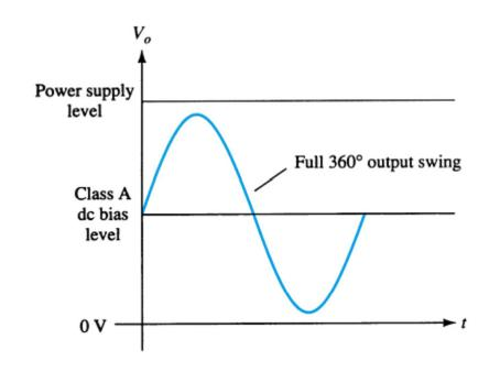
Remember that the DC load line indicates the maximum and minimum limits set by the DC power supply.
