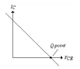
The Q-point is at 0V on the load line, so that the AC signal can only swing for one-half cycle.
